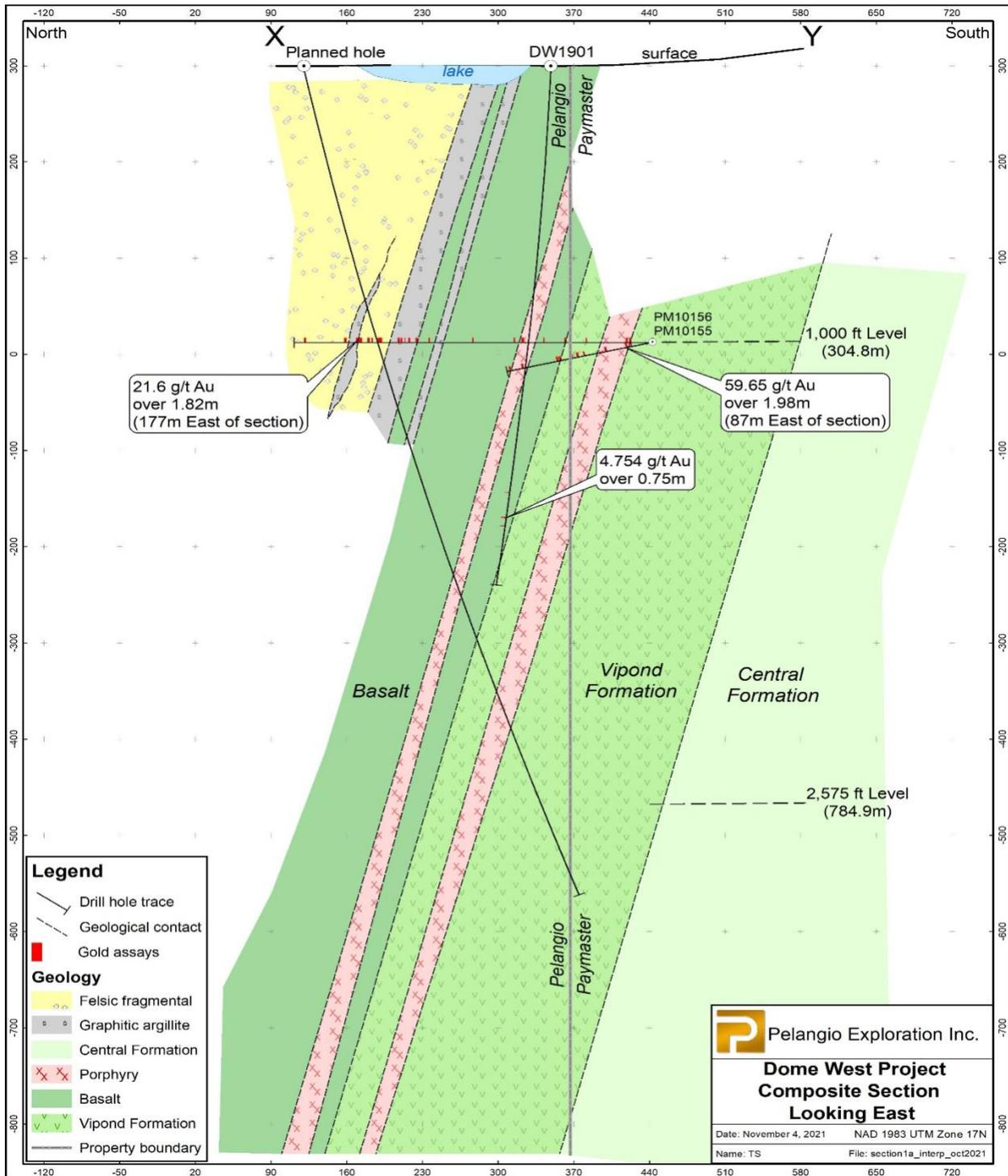
Figure 4: Historical Composite Level Plan with Geology
