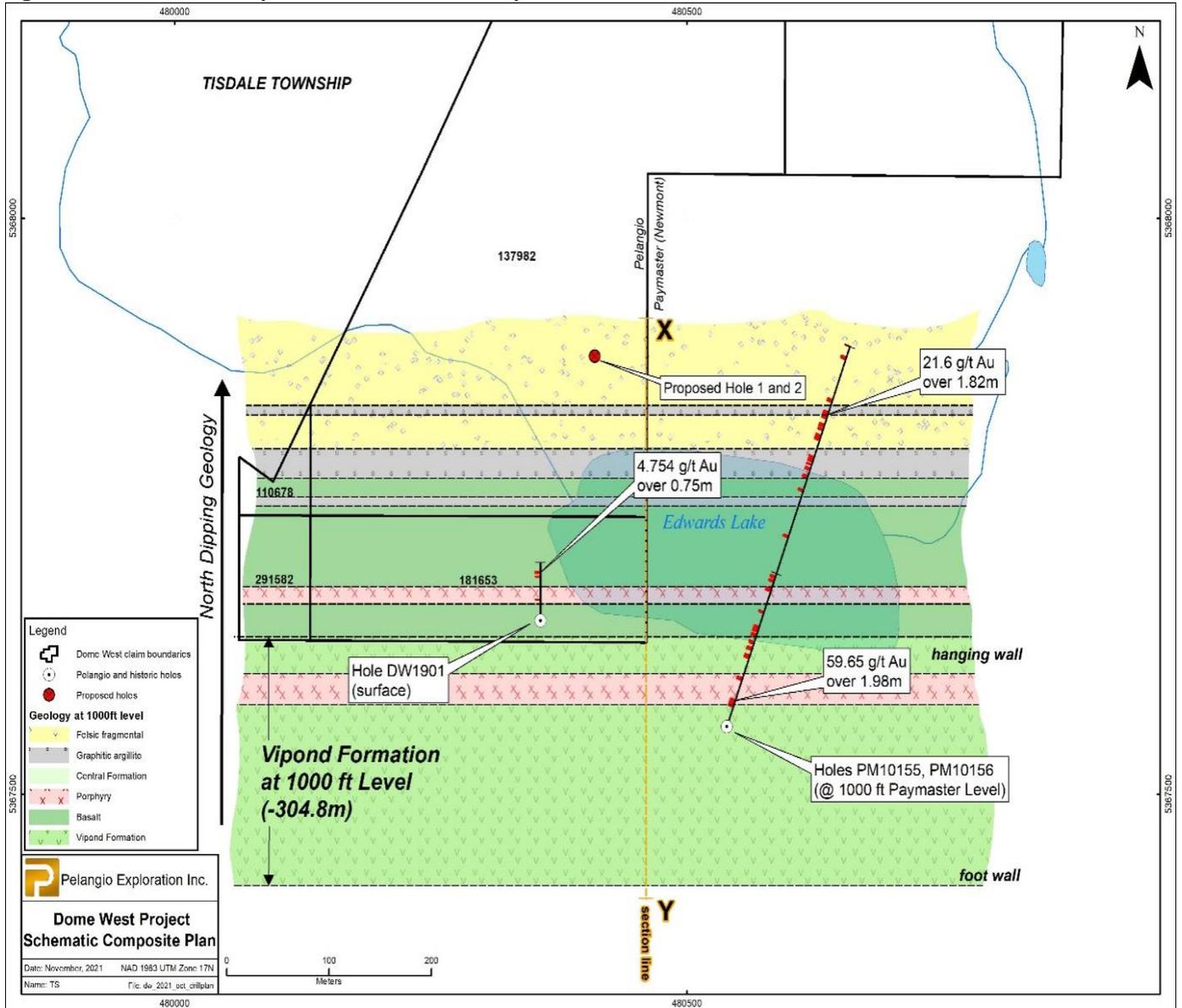
**Figure 3: Dome West Schematic Section**
