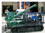
Low Environmental Impact 'Grasshopper' Drill Rig
