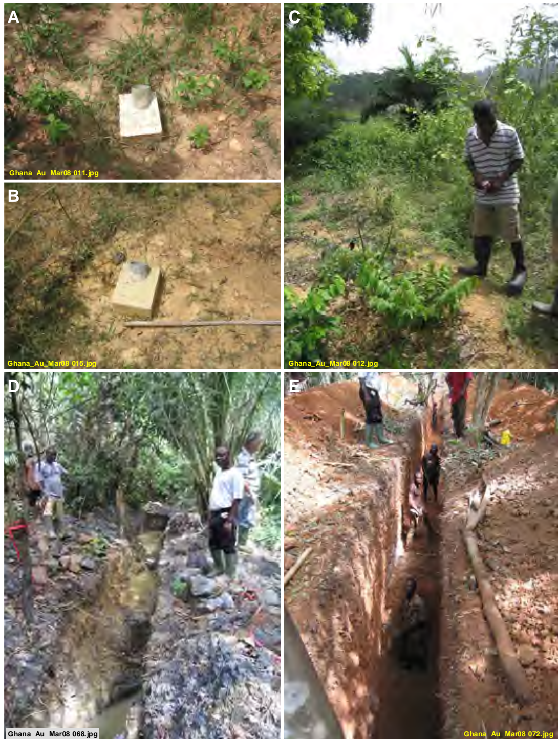
Figure 20. A-B. Benchmark for Boreholes PG07-KU-04 and KU-02 Drilled by Pelangio on the Kusa Target, Meduma Concession. C. Backfilled Trench at Kusa. D. North-trending Trench on Copper West Target. Silica Rock Grading 1-5 gpt Gold, Kyereboso No.2 Concession. E. New Trench Recently Excavated at the New House Trench Area to Follow-up on Trench Results.
